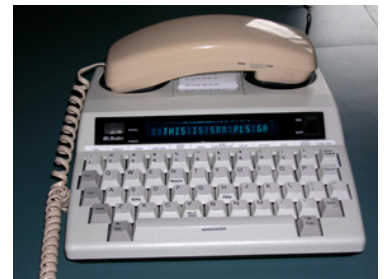
TTY with Telephone
